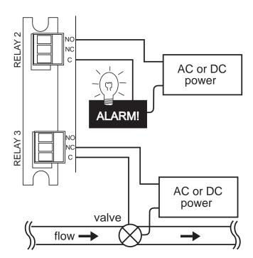
NO = normally open (closes when energized) NC = normally closed (opens when energized)
